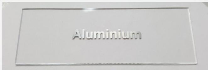
*Photo: Laser-induced PVD-marking, showing “Aluminium” on glass*
