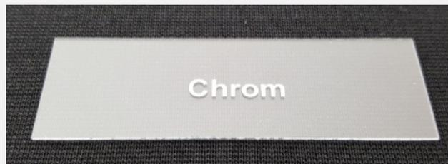
*Photo: Laser-induced PVD-marking, showing “Chrome” on glass*
