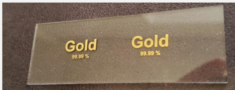
Photo: Laser-induced PVD-marking “Gold 99,99 %”, applied on the upper side (left) as well as on the backside (right)
