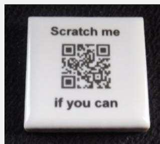
*Photo: Laser-induced PVD-marking, showing a QR-code*
