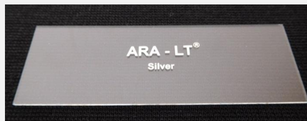
Photo: Laser-induced PVD-marking on glass, showing a silvery text
