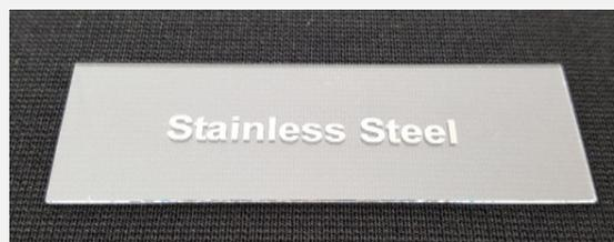
*Photo: Laser-induced PVD-marking, showing “Stainless Steel” on glass*
