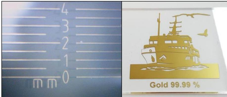
*Figure 2: Laser-applied gold lines (left) and a golden boat (right)*
