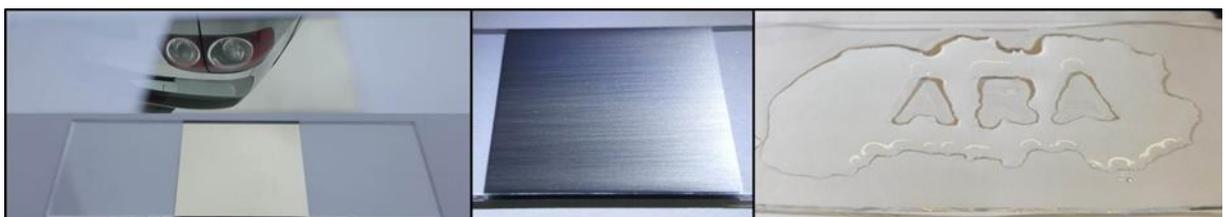
*Figure 2: Laser-applied silver mirror (left), brushed steel surface (middle) and selective easy-to-clean coating (right)*
